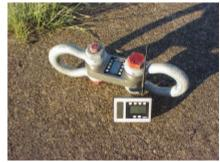
via a radio remote readout. The values reported in the raw data represent the drag factor as calculated by the force divided by the weight of the test unit for the relative percentage in relation to gravity for the µ value. Two semi trailers and the school bus were slid on their sides, and the automobile was slid on its roof.
